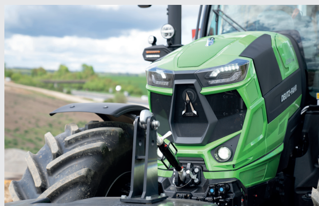
↑ LED driving lights and characteristic LED worklights.
