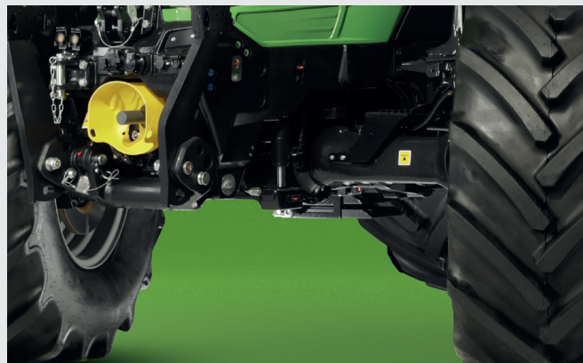
↑ Front suspension concept with high ground clearance and 3 adjustable levels inside the InfoCentre PRO .
