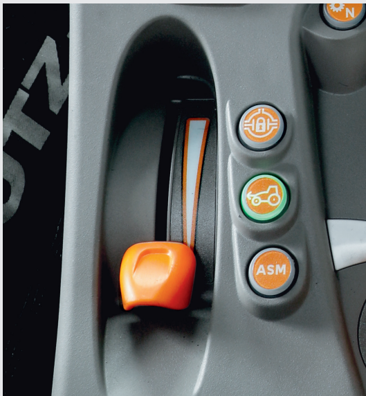
↑ Independent hand throttle and electrohydraulic activation of differential lock, all-wheel drive and ASM automatic function.
