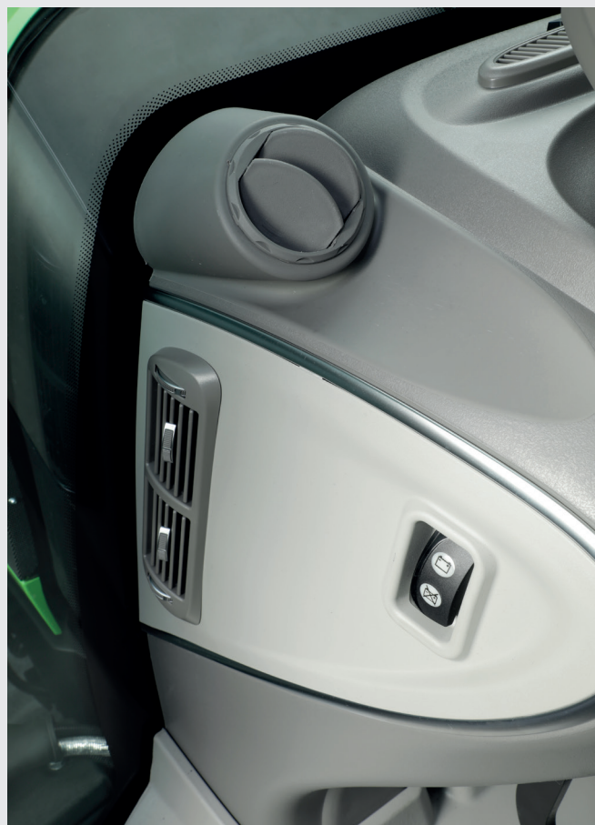
↑ Additional air outlets and battery main switch comfortably placed in the cabin.
