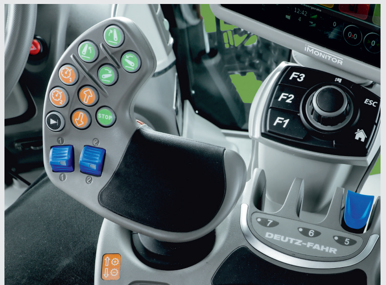
↑ Ergonomic MaxCom joystick with front and rear lift, engine, transmission, headland management and two two proportional hydraulic valve control units.
