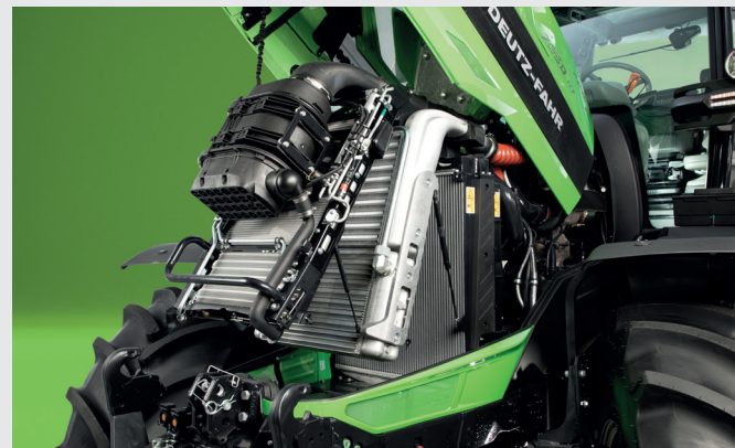
Aluminium cooling system with one-hand access lever and Powercore air filter.
