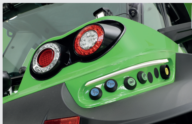
↑ Fender controls on both sides illuminated with LED light bar.
