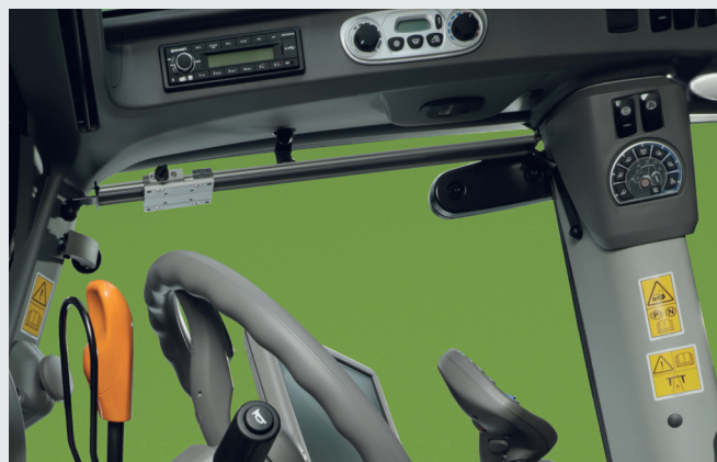
↑ Adjustable monitor support rail.
