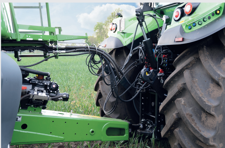
↑ Rear linkage in transport position for less interference with drawbars while cornering.
